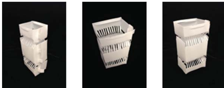
FIGURE 1. Custom-fabricated Teflon coverslip rack. Our coverslip racks hold 13 glass coverslips (22 × 60 mm) with minimal contact and four units can be linked together to clean and silanize 52 coverslips in one preparation. Teflon can withstand all the chemicals used in the protocol and the racks can be reused for several years.
